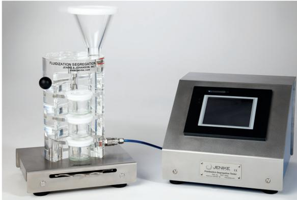
The Jenike Fluidization Segregation Tester measures the tendency of a powder to segregate when fluidized.
