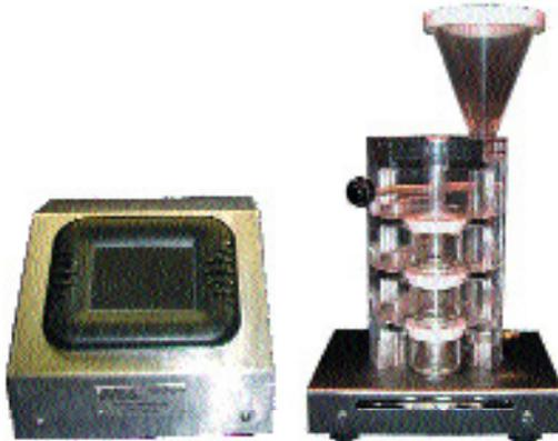
the sample contained within each section to drop into its appropriate collection cup. This unique design provides fast, easy sample collection.
